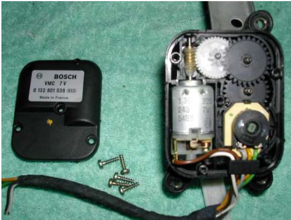
Internals of a flap motor – in this case the temperature flap one. Position sensing potentiometer is bottom right
