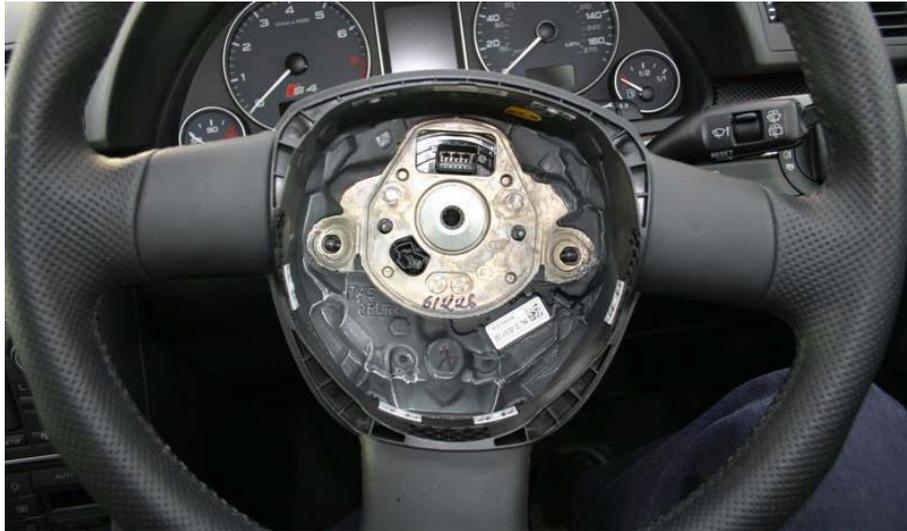
18. Reconnect the airbag wiring harness and refit the airbag by screwing the airbag back in place and put back the small plastic clips at the back of the steering wheel.
