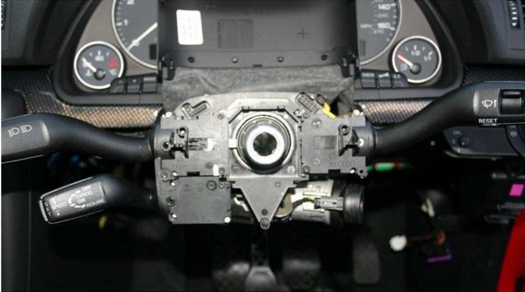
14. Reconnect the slip ring and connect the wiring harness, reconnecting all 3 clips.
